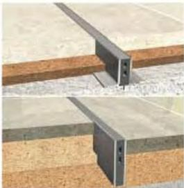
**AFE EE Movement Joint Systems** are designed in floors and walls where movements are anticipated. They are suitable for use with ceramic, terrazzo, marble and similar floor finishes. The systems provide edge protection and an impervious, maintenance free joints. Our Joint system comprises of a compressible polychloroprene core, sandwiched by brass, stainless steel or aluminium side plates.
