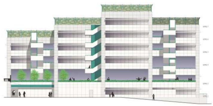
Also under the original design, the designers proposed lustre wall tiles arranged in a clearly defined grid. Time and cost considerations led to changes in materials, however, and textured spray paint was later applied instead of tiles to the exterior while retaining the grid and line detailing. Soft pastel colours are used for the four classroom wings — primary colours and the like would have looked too youthful for this project.
