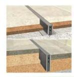
AFE EE Movement Joint Systems are designed in floors and walls where movements are anticipated. They are suitable for use with ceramic, terrazzo, marble and similar floor finishes. The systems provide edge protection and an impervious, maintenance free joints. Our Joint system comprises of a compressible polychloroprene core, sandwiched by brass, stainless steel or aluminium side plates.
